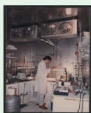
張宏君教授於實驗室純化藍白蛋白。由於蛋白質具有熱不穩定，故實驗多常長時間在4°C低溫房中進行。 Professor Zhang Yexun laboratory purification of proteins. As the protein perishable, it will take time and more experiments carried out at 4 °C cold room.
